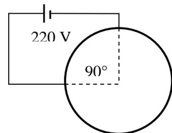
20. A wire of resistance  $R$  is bent in the form of a circle and is connected to a 220 V source as shown (Above, Right). If the energy provided by the source in 42 s is same as the energy required to raise the temperature of 11 kg of water through  $44^\circ\text{C}$ , find the value of  $R$ .
